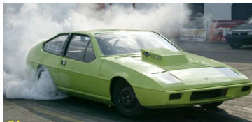
Mark Evans' 1976 Eclat, equipped with 5 litre Chevrolet engine
