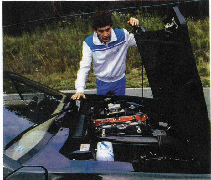
Ayrton takes an expert look at the S.E.'s power unit before his test and sees twin overhead camshafts under the red cam covers.
